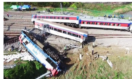
Yulchon Station derailment accident ('16.4), train driver ignored speed limit
