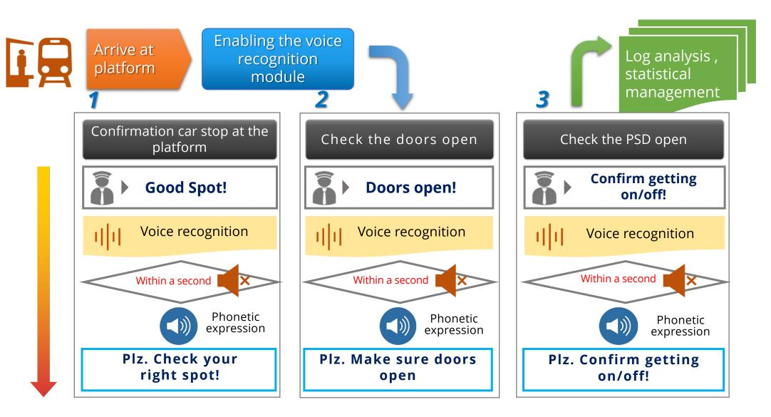
✓ After ending of the process, goes into dormant state. If the train gets next station, the above procedure starts all over.
