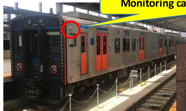
Monitoring camera on the driver's cab
