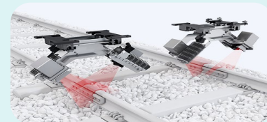
Joint Bar inspection
