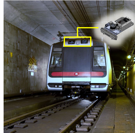
Train-borne Railway Infrastructure Inspection System
