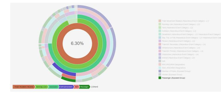
Examples of ARRM outputs, the first one showing the risk profile for infrastructure manager risk (in fatalities and weighted injuries per year) vs rolling stock operators. The second one shows the overall proportion of passenger risk coming from rolling stock collision on running lines (as 'owned' by infrastructure managers).
