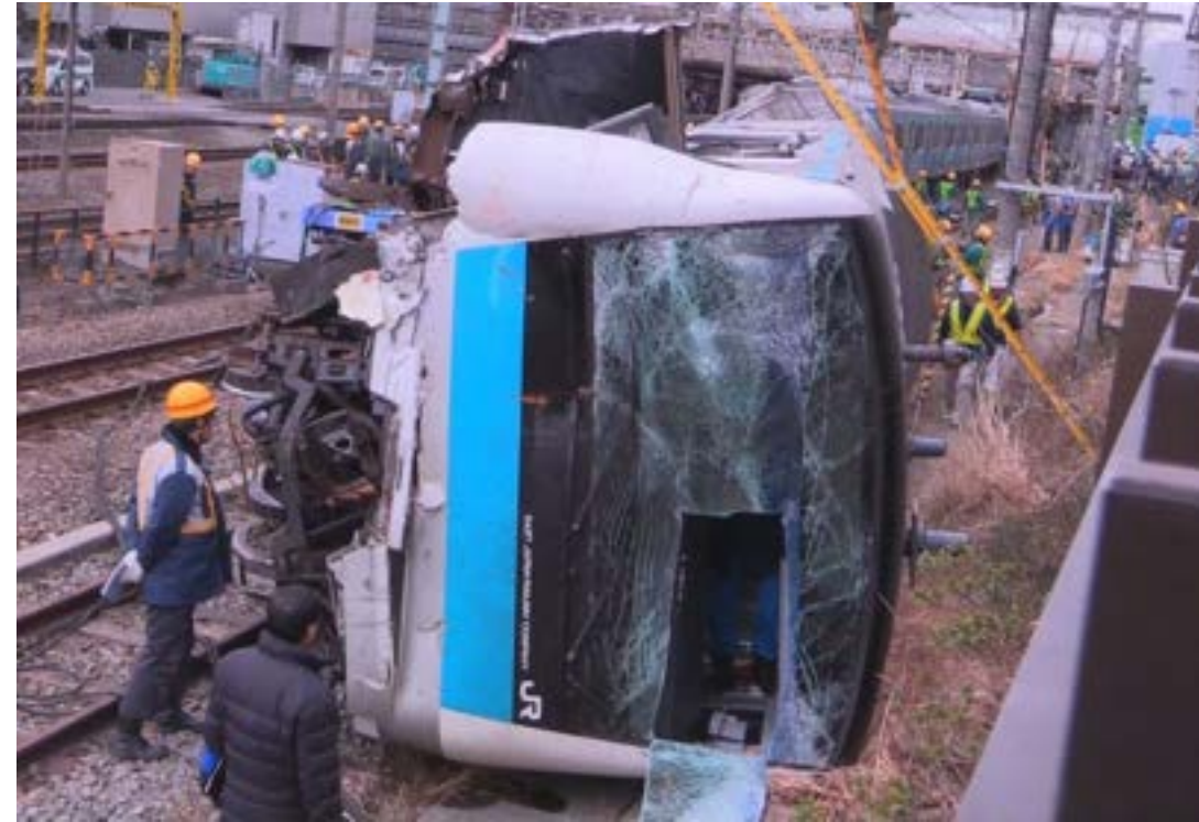
In the train derailment accident on the Keihin-Tohoku Line (February 23, 2014), a road vehicle for construction work entered a track that was not closed, causing a collision and derailment of a traveling train.
