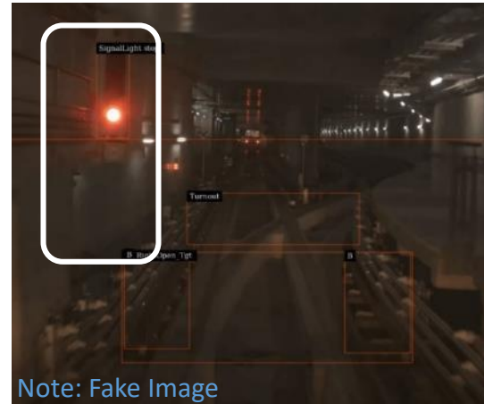
Early warning of stop signal, SPAD alarm if stop signal is passed
