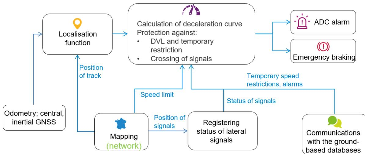
The ESVE+ system, which is currently in the prototype phase, will make it possible to monitor the risks of trains exceeding the speed limit of the particular line (at a lower cost than ERTMS while waiting for its deployment), thanks particularly to the following functions:
