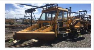
Manufacturer's rated axle loads not provided in checklist (shown only as PASS). Rear axle back-to-back dimension is outside tolerance (1522 vs. 1523).
