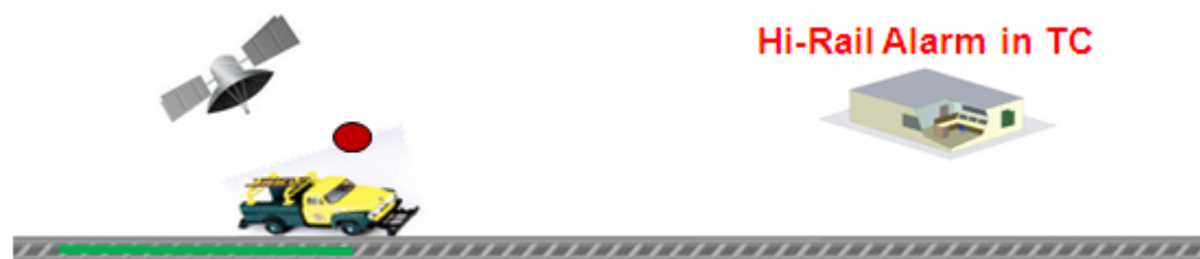
Figure 5: Hi-Rails – position tracking and alarms.
