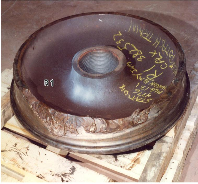
**Photo 2: Shattered Wheel from a Different Incident (but same wheel manufacturer)** Source: TSB Report R04T0008
