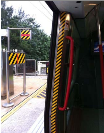
Figure 8: Vertical stopping mark on the East Rail Line
