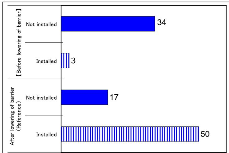
**Figure 1: The relation between existence of obstacle detection device and accident number**
