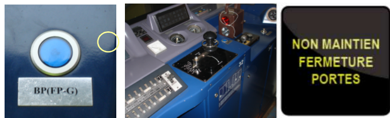
Figure 1. BP FP-G and “doors not locked” warning light.
