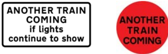
Figure 2: Sign (left) and light signal (right) advising road users that another train may pass through the crossing
